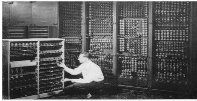
Replacing a bad tube meant checking among ENIAC's 19,000 possibilities. 2020/3/12
